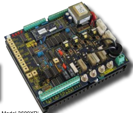
Model 3600XRI Up to 32 amps - 6.9"x 8"x 3.2" (175x200x80 mm) 36 amps unit - 6.9"x 8"x 3.8" (175x200x95 mm)
